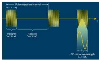
Radar operates by transmitting pulses of electromagnetic energy and detecting the backscattered energy by listening during the time between pulse transmissions.
