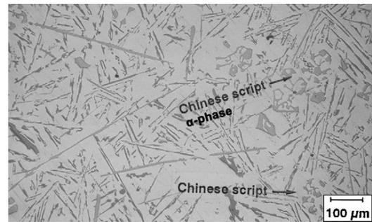
Fig. 5. Microstructure of the Mn-modified alloy containing 1.4 per cent Fe.
