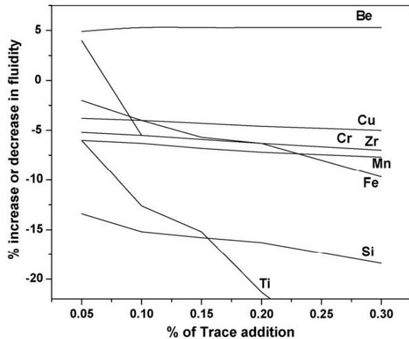
Fig. 1. The effect of trace addition on fluidity of pure aluminium.
