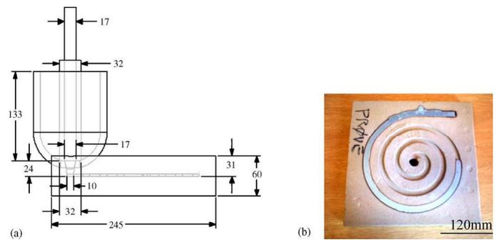
Fig. 2. The experimental setup for fluidity test.
