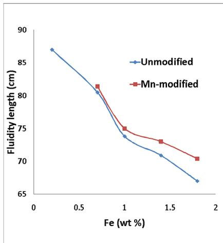
Fig. 3. The effect of Fe on the fluidity of un-modified and Mn-modified alloys.
