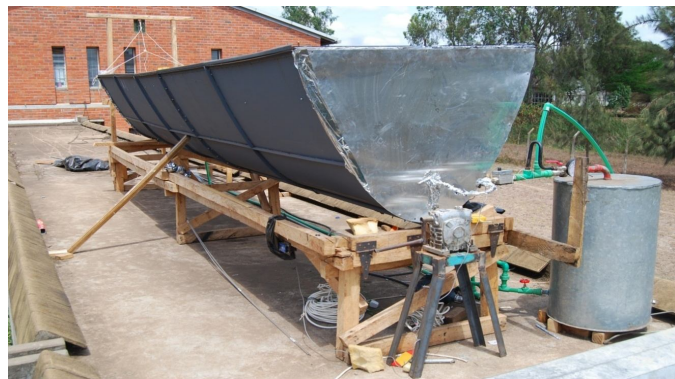
Fig. 1. Fabricated prototype parabolic trough solar concentrator for steam production.
