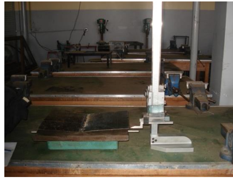
Figure7: Distortion of the welded plate
