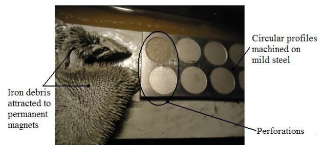
Fig. 6: Debris separation mechanism from dielectric fluid using magnetic forces.
