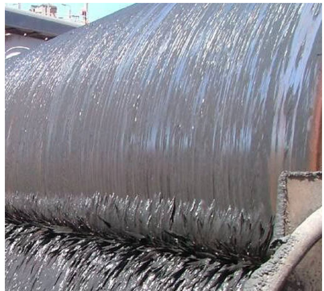
Fig. 4: Typical dense media magnetic separator.
