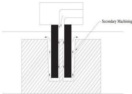
Fig. 3. Effect of secondary discharge machining
