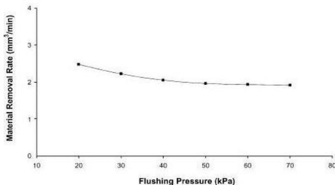
Fig. 6. Effect of flushing pressure on material removal rate [11]
