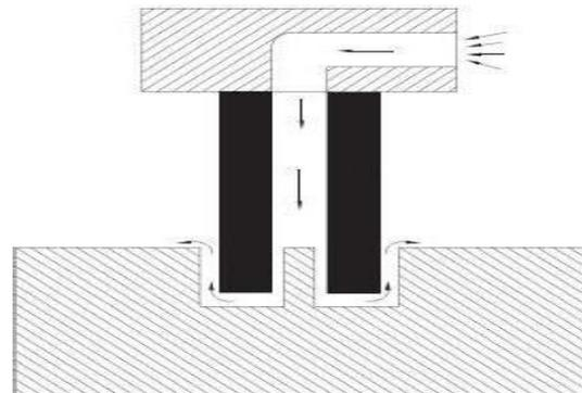
Fig. 1. Pressure flushing through the electrode
