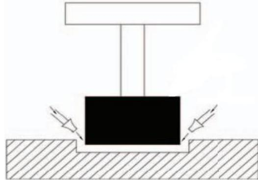
Fig. 4. Effect of secondary discharge machining
