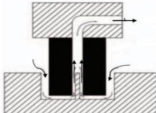
Fig. 5. Suction flushing
