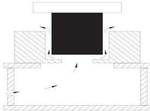
Fig. 2. Pressure flushing through the workpiece
