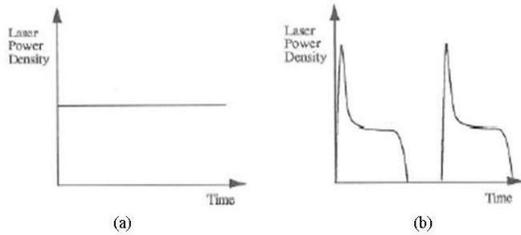
Fig. 2. Laser beam temporal modes(a) continuous wave (b) pulsed mode [6]
