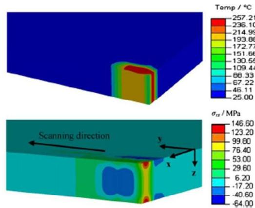
Fig. 6. Simulation results showing temperature and stress distribution across the thickness at the leading edge of glass at 0.2s along the scanning direction. [16]
