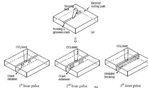
Fig. 3. pulsed laser breaking process of (a) diamond scribing and (b) laser breaking [15]
