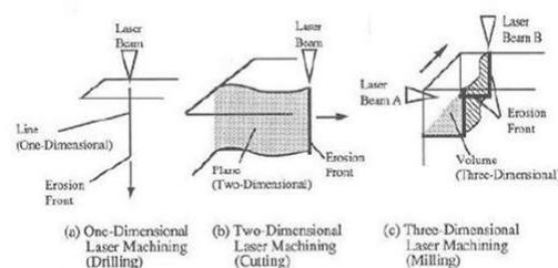
Fig. 1. Schematic showing one, two and three dimensional laser machining [6]
