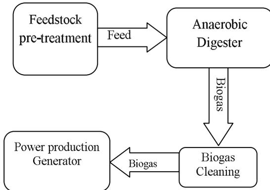
**Figure 1 Biogas Production Sequence**
