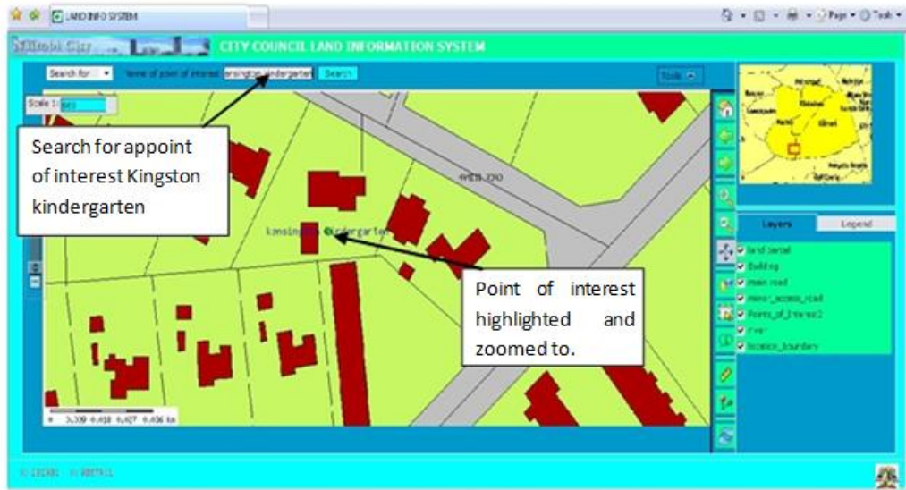
Figure 10: Using a point of interest to navigate to a land parcel of interest
