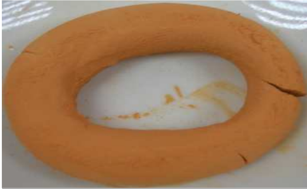
Figure 2: Effect of grain size on the strength of clay particles at 25 \mu\text{m} and temperature (800°C) after firing for five hours
