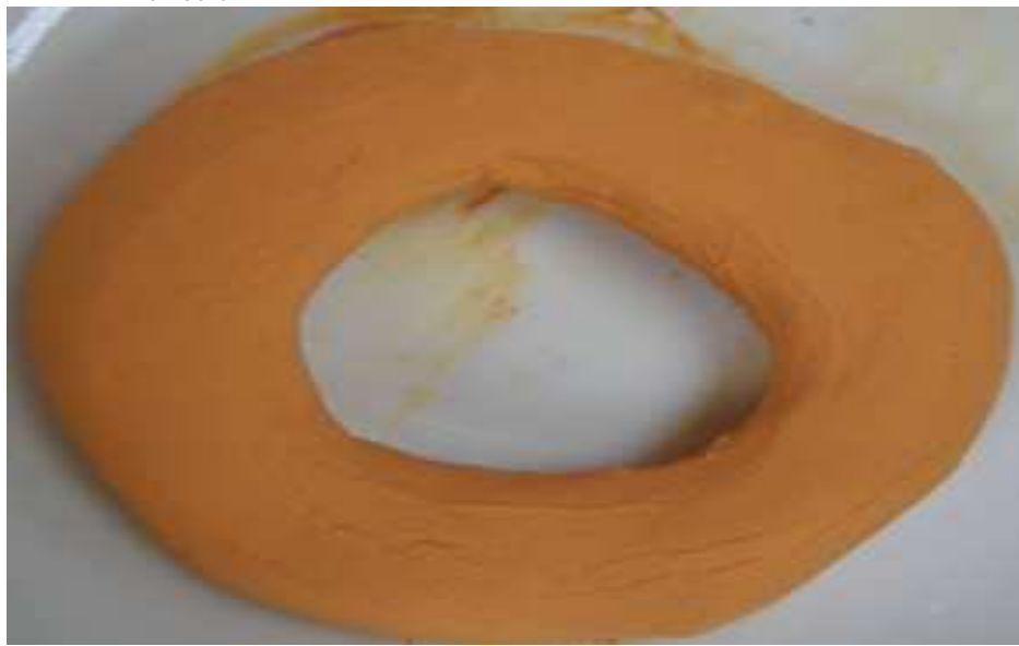
Figure 2: Effect of grain size on the strength of clay particles at 25 \mu\text{m} and temperature (800°C) after firing for five hours
