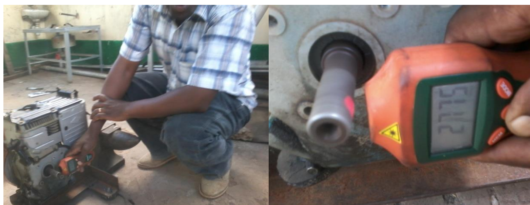
Fig 3: measuring the shaft speed of a gas driven engine using a digital tachometer.
