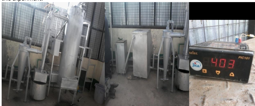
Fig. 1: The gasifier equipment used in the test and the temperature monitoring meter
