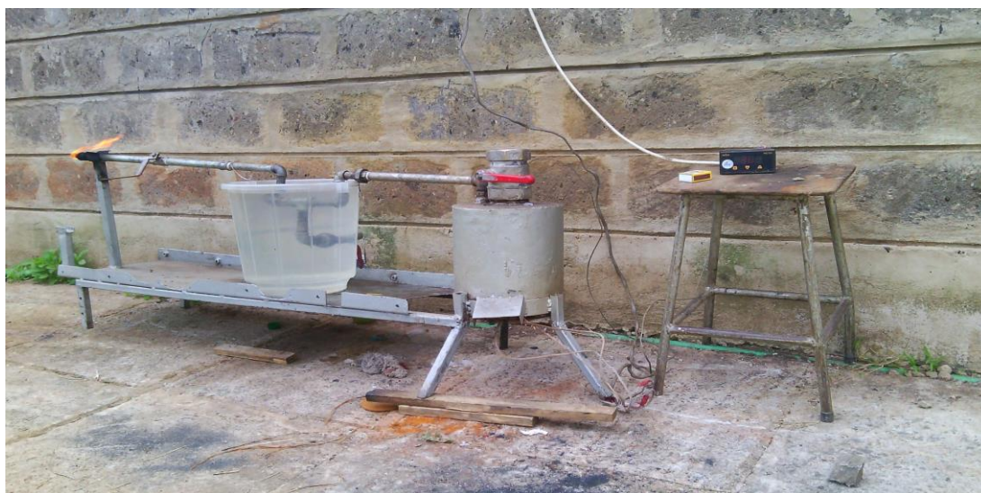
Plate 1: Pyrolysis batch reactor used for oil production
