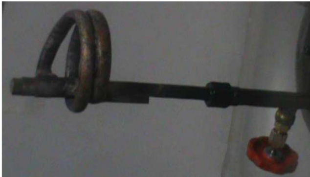
Figure 6: Modified Lamp Vapourizer
