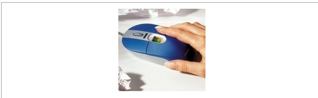
Figure 2: A computer mouse with a built-in fingerprint scanner Photo courtesy: Siemens
