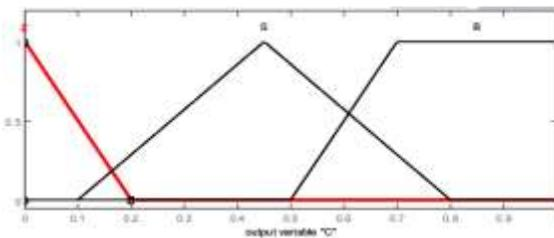
Fig. 8: Membership functions of the output variable C
