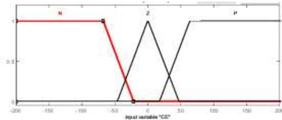
Fig. 7 Membership functions of the input variable CE
