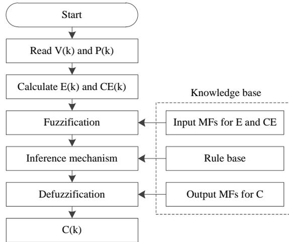
Fig. 5: Flowchart of the fuzzy-based adaptive step-size algorithm.
