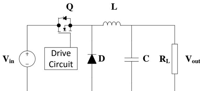
Fig 3: A circuit diagram of a buck converter
